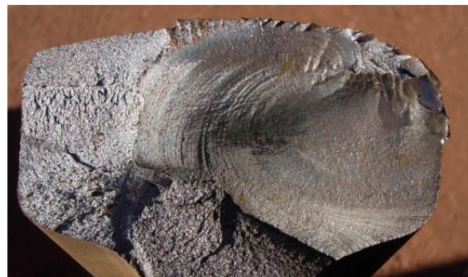
Figure 4: Transverse defect that developed from gauge corner cracking.
